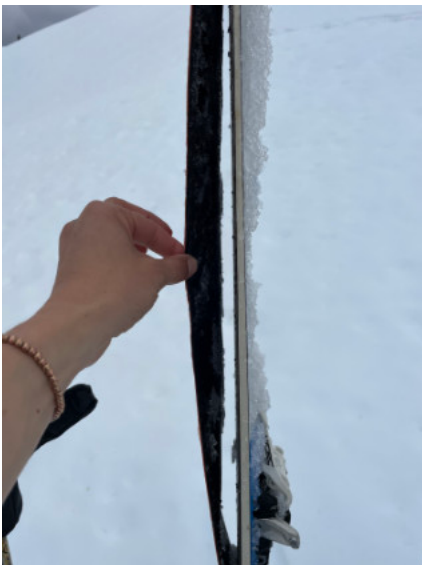
Total glue failure!
