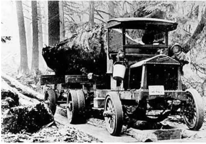
Logging truck on a wood "fore and aft" logging road. PHOTO SOURCE UNKNOWN
