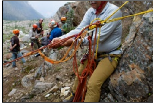
Cyril Shokoples showing us a pulley system for raising an injured climber up to you.
